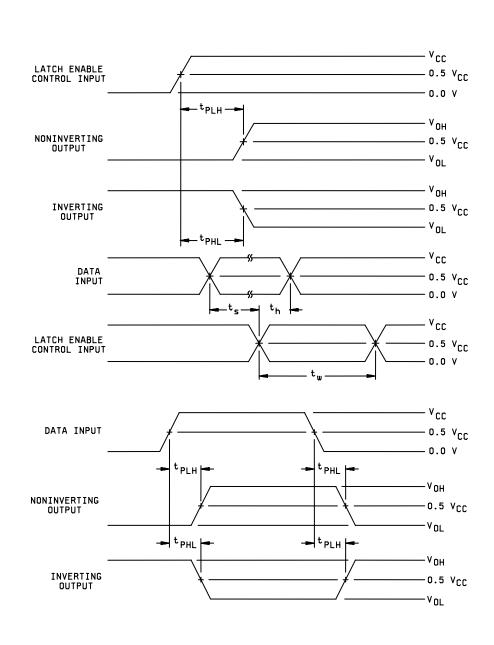
FIGURE 5. Switching waveforms and test circuit.
