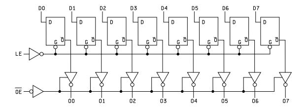
FIGURE 3. Logic diagram.
