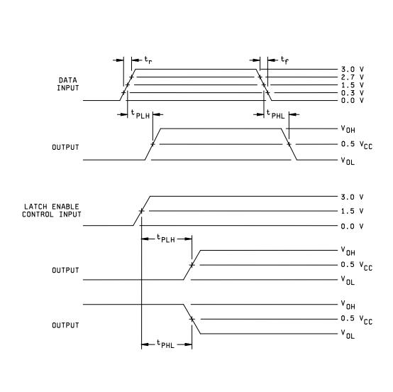
FIGURE 5. Switching waveforms and test circuit.
