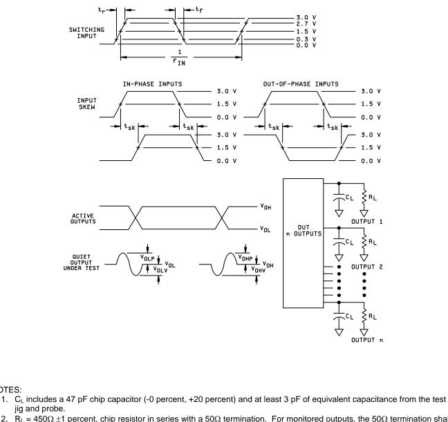
2.  $R_L = 450\Omega \pm 1$  percent, chip resistor in series with a 50 $\Omega$  termination. For monitored outputs, the 50 $\Omega$  termination shall be the 50 $\Omega$  characteristic impedance of the coaxial connector to the oscilloscope.
