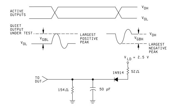
NOTE: Resistor and capacitor tolerance =  $\pm 10\%$
