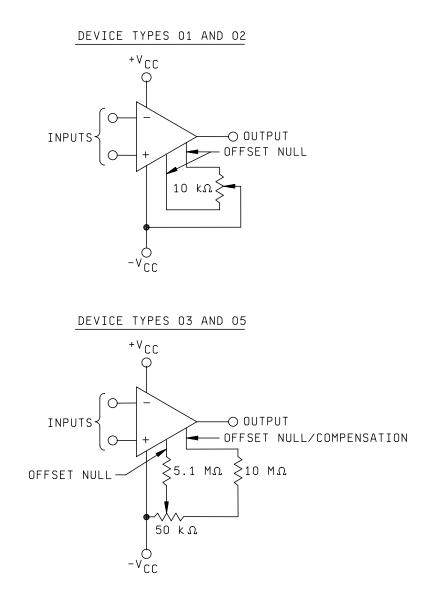
FIGURE 2. Offset null circuits.
