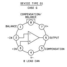
Figure 1. Terminal connections and logic diagram.
