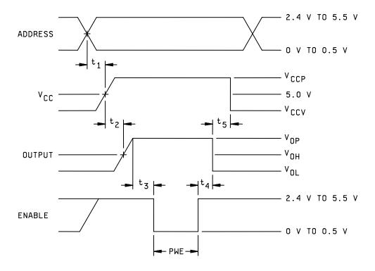
FIGURE 5d. Programming voltage waveforms during programming for circuit G.
