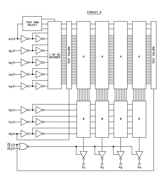
A = 32 x 8 Memory Array B = 1 of 8 Decoder
