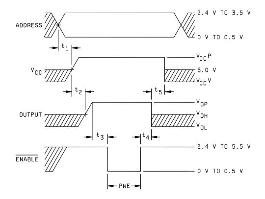
FIGURE 7g. Programming voltage waveforms during programming for circuit G.
