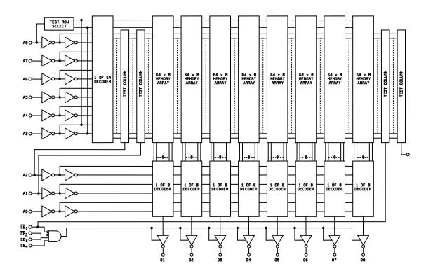
FIGURE 5. Logic diagrams.
