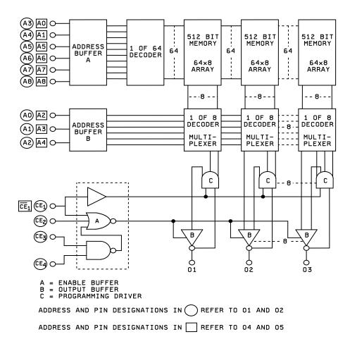
LOGIC CIRCUIT C (Device types 01 and 02) and LOGIC CIRCUIT H (Device type 02)
