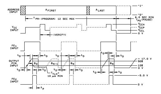
NOTE: All other waveform characteristics shall be as specified in table IVC. FIGURE 7c. <u>Programming voltage waveforms during programming for circuits C and H.</u>
