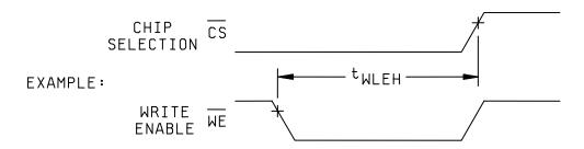
The example shows Write pulse setup time defined as t<sub>WLEH</sub>-time from Write Enable to low to Chip Enable High.
