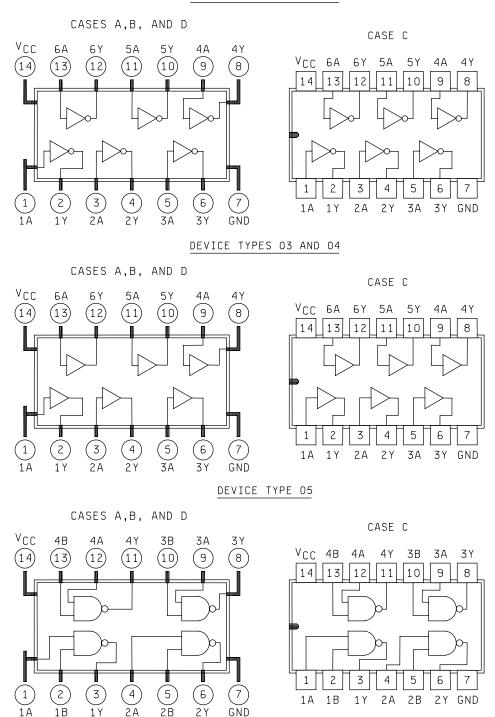
Figure 1. Logic diagram and terminal connections (top views).
