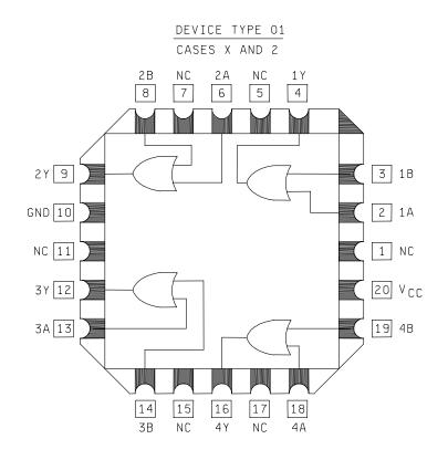
FIGURE 1. Terminal connections and truth table.
