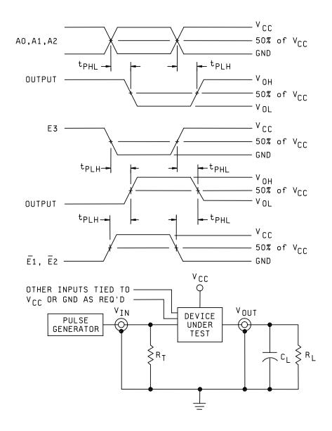
FIGURE 3. Switching waveforms and test circuit.
