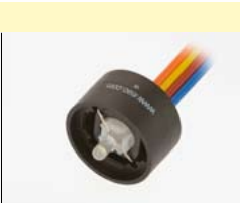
Switching element, 24VDC, IP67; ribbon cable 300 mm, four strands, 1NO
