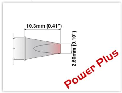
EBM7CH175H Chisel 30° 2.5mm (0.10"), Power Plus
