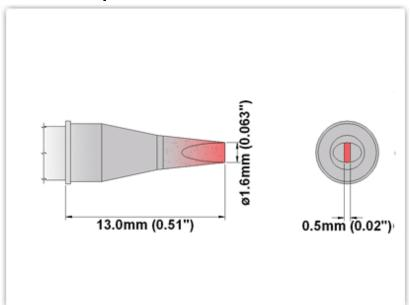
EP75CH016 Chisel 30° 1.60mm (0.06")
