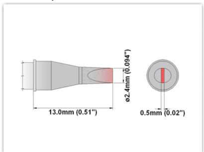
EP75CH024 Chisel 30° 2.40mm (0.09")
