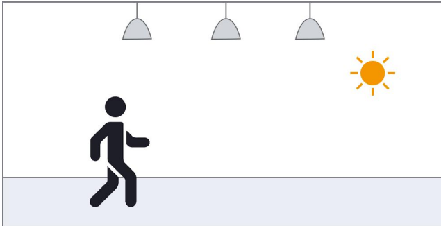
The light does not trigger on when detect moving object with the ambient brightness is enough
