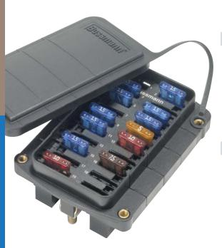
The Rear Terminal ATC® Fuse Panel (RTA) is a rear-fed panel with high component retention, which makes it an ideal choice for high vibration environments including construction, agriculture, bus, RV, heavy trucking equipment, etc. It is available in multiple lengths and internal bussing configurations. This allows for up to three separate power input circuits and 32 individual output circuits.
