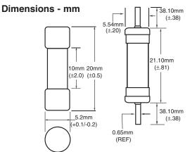
· With TR2 packaging code, lead wire length is 19.05mm
