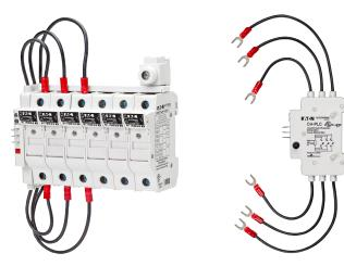
The Bussmann series resettable PLC fuse monitor permits easy integration with a Programmable Logic Controller (PLC) or other monitoring and control equipment. Signals up to three-phases. Includes 0.11" (2.8 mm) quick-connects for power, signal and ground connections.
