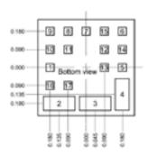
Projection: Third angle projection Tolerance:  $\pm$  0.01 Pad 1&5~12 = 0.04 × 0.04 Pad 2~4 = 0.07 × 0.157
