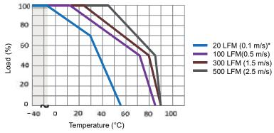
The derating curve was measured at 12 V input and 5 V output.
