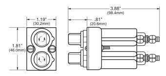
Drilled Mounting Hole Dimensional Tolerance ± 0.005" (0.13 mm)
