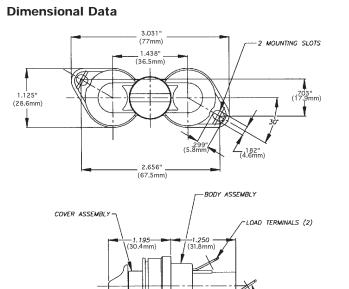
Catalog Symbol: HPS2 Description: Meets requirement of UL 1598 that both poles be removed simultaneously. Fuse Type: 13/32" x 1-1/2" Agency Information: UL 512 Recognized, (Guide IZLT2, File E14853) CSA Certified: (Class 6225-01, File 47235) Flammability Rating: 94V-0 Terminals: 1/4" guick connect / solder
