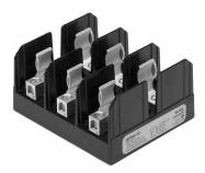
Catalog Symbol: J70100 Ampere Rating: 100A Voltage Rating: 700Vac Agency Information: UL Recognized, Guide IZLT2, File E14853 Withstand Rating: 200,000 RMS Sym. Amps For use with 22 × 58mm fuses (FWP-40A22F, FWP-100A22F, etc.) Materials: Thermoplastic UL Flammability: 94VO
