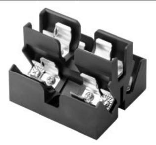
Catalog Symbol: JP Series Pyramid Style Fuseblock Ampere Rating: 30 Amperes Voltage Rating: 600 Volts Withstand Rating: 200,000 RMS Sym. Amps Agency Information:
