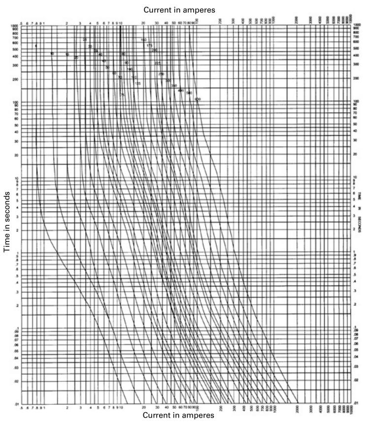
Time-current characteristic curves – average melt 600V RES (LKS Fuse links)
