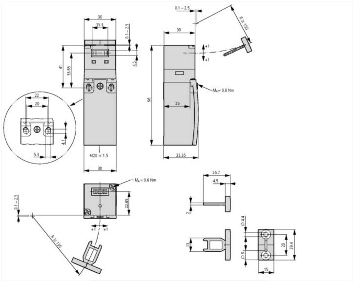
Switch must not be used as a mechanical stop Terminal marking according to EN 50 013
