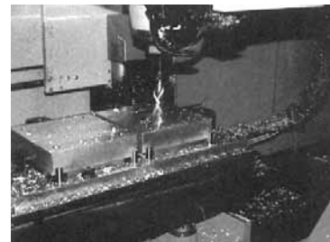
An Inductive Proximity Sensor Monitors Drilling Operation
