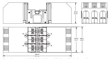
3-pole ganged 200 A holder with installed shroud
