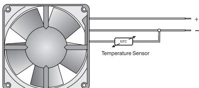
The temperature sensor for controlling the motor speed is not included in the scope of delivery.
