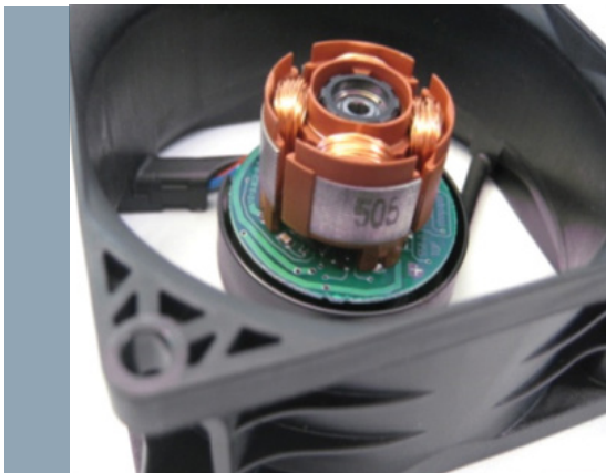
*IP20 protection - for indoor (clean/dry) applications where no additional protection for motor (electronics or windings) is required.
