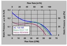
The diagram shows the best of the measured competitive models. The AC 100 NR is slightly superior to the best model. In the speed version H with 4500 min<sup>-1</sup>, the fan performance is considerably higher.
