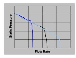
The constant volume regulation assigns a defined flow rate within a pressure range. The fan automatically adapts its discharge rate to environmental changes, e.g. filter, wind pressure and obstacles. As the fan only operates with the power that it actually requires to fulfil its task, it is extremely energy-saving and quiet when operating in continuous mode.
