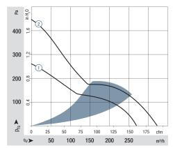
Air performance measured according to: ISO 5801. Installation category A, without contact protection. Noise: Total sound power level  $L_WA$  ISO 103002 measured on a hemisphere with a radius of 2 m. Sound pressure level LpA measured at 1 m distance from
