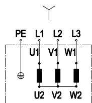
Change of rotation direction by reversing two phases
