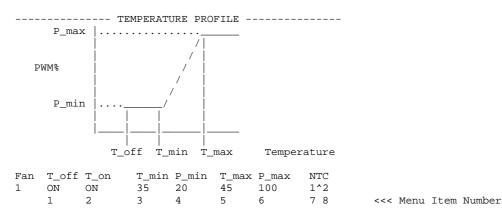
Type "7" to change the NTC Thermistor 1 used setting.
