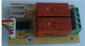
The interface used is compatible with the ebm-papst "EC Matrix" control bus, support for other EC-Matrix boards possible, contact ebm-papst.
