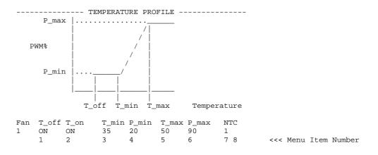
Type "5" to change the Temperature at the Top of Proportional Control Band, display will be as shown:
