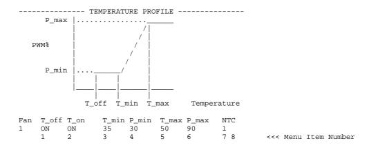
Type "4" to change the PWM Output at the Bottom of Proportional Control Band and below, display will be as shown:
