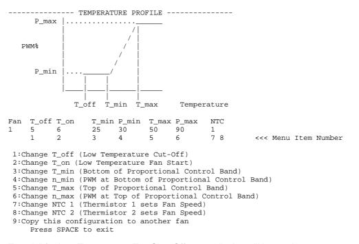
Type "1" for Low Temperature Fan Shut-Off menu, display will be as shown:
