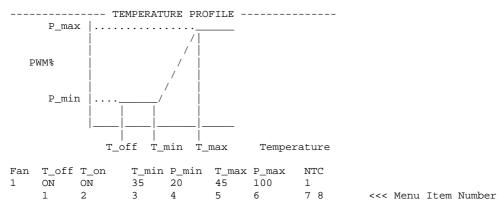
Type "8" to change the NTC Thermistor 2 used setting, if both thermistors selected then speed will be set by whichever of NTC Thermistor 1 or NTC Thermistor 2 is hottest. Display will be as shown:
