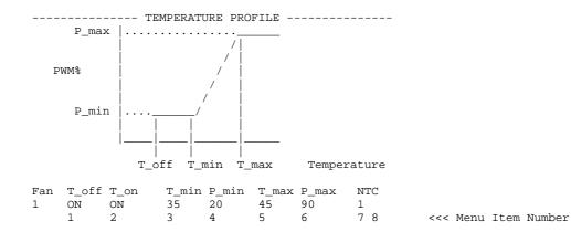
Type "6" to change the PWM Output at the Top of Proportional Control Band and above, display will be as shown:
