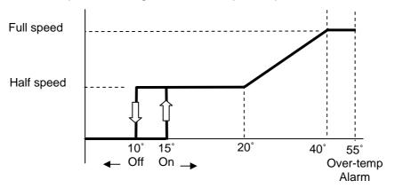
Each fan may have a different profile using either thermistor as configured. The fans can be set to switch off at low temperature, programmable option, individually programmable on and off points.
