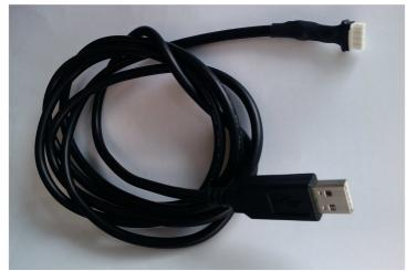
ebm-papst part number 210-HAR11887, type A USB to TTL serial data adapter, length 1.8m. Connects TMS to PC for configuration and data logging.
