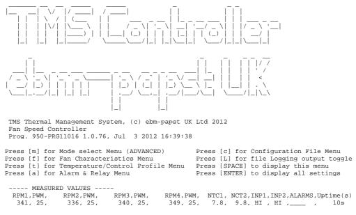
To display the full configuration, press the [Enter] key on the PC keyboard To display the configuration menu and measurement header, press [space].
