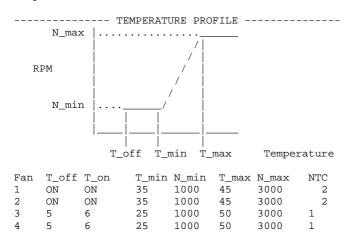
In this operating mode the Controller output sets the fan RPM (Closed Loop control). The fan speed control PWM output will be continuously adjusted to bring the measured fan RPM to the set value.
