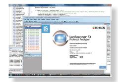
The LonScanner FX Protocol Analyzer is an easy-to-use Windows tool that lets manufacturers, system integrators, and end users observe, analyze, and diagnose the behavior of LonWorks<sup>®</sup> networks. It provides the advanced productivity features common in data network analyzers, adapted to the unique needs of control networks.
