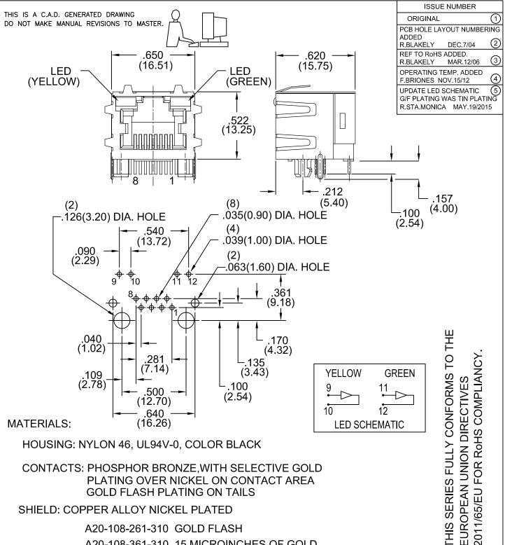
CONTACTS: PHOSPHOR BRONZE, WITH SELECTIVE GOLD PLATING OVER NICKEL ON CONTACT AREA **GOLD FLASH PLATING ON TAILS**
