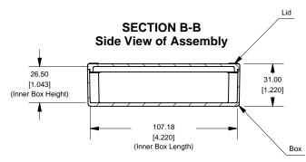
Enclosures can be Factory Modified (Milling, Drilling, Printing etc.) Solid models of this enclosure available in STEP or IGES.
