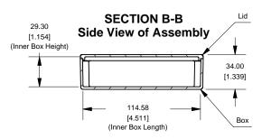
95.00 [3.740] 120.00 [4.724] Enclosures can be Factory Modified (Milling, Drilling, Printing etc.) Solid models of this enclosure available in STEP or IGES.
