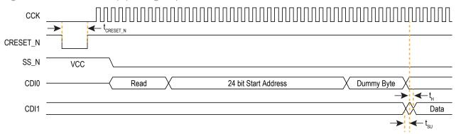
Figure 11: SPI Passive Mode (x1) Timing Sequence
