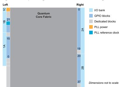
Figure 13: Floorplan Diagram for BGA49 and BGA81 Packages
