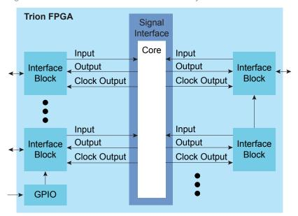
Figure 6: Interface Block and Core Connectivity
