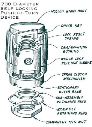
**Push-to-Turn:** Knob design utilizes sprag-type clutch mechanism offering security against shock, vibration and inadvertent change while providing ease of operation, accurate positioning and positive locking.
