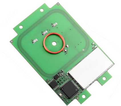
TWN4 MultiTech 2 LEGIC M PCB top view (exemplary)
