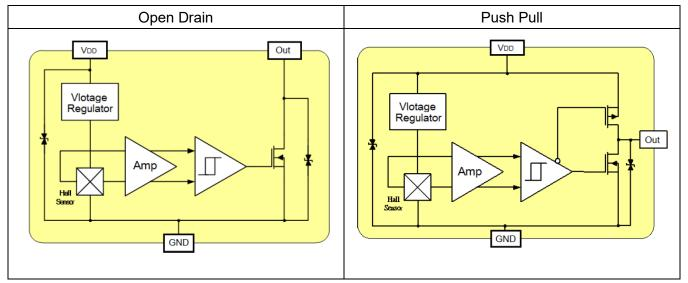
Note: Static sensitive device; please observe ESD precautions. Reverse VDD protection is not included. For reverse voltage protection, a  $100\Omega$  resistor in series with VDD is recommended.
