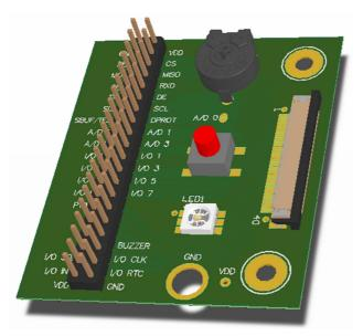
Note: Illustration shows a fully assembled pcb including optional components. Some components are not assembled ex factory.
