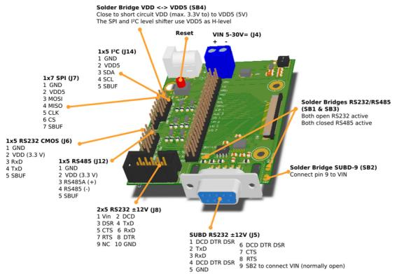
Note: Illustration shows a fully assembled pcb including optional components. Some components are assembled ex factory.
