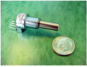
The Electroswitch 500 Series Magnetic Encoders are built upon a contact free integrated circuit design. This encoder integrates Hall Effect sensing and digital signal processing to provide high-resolution angular measurement solutions.
