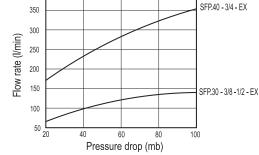
(difference between the pressure inside and outside the reservoir)
