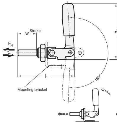
\* Complete with type index of the push-pull type toggle clamps
