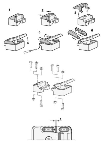
Prior to installation remove the slam latch cover as shown in the sketch. Socket head cap screws DIN 912, hexagon head screws DIN 933 and hexagon nuts ISO 4032 each with thread size M 6 can be used for mounting the slam latch. After installation the covers are reassembled in reverse order. The covers cannot be removed when the slam latch is closed and consequently protect against vandalism.
