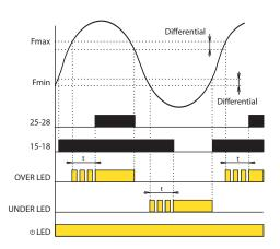
After the supply (monitored) voltage is connected, the green LED is on. If the value of the monitored frequency falls within the range between the two set levels Fmin - Fmax no red LED is on. The relay UNDER is triggered (contacts 15-16-18) and the relay OVER is disconnected (contacts 25-26-28).
