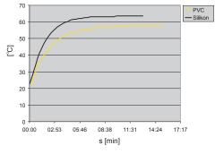
PVC - reaction to water temperature from 22.5 °C to 58 °C (from 72.5 °F to 136.4 °F).
